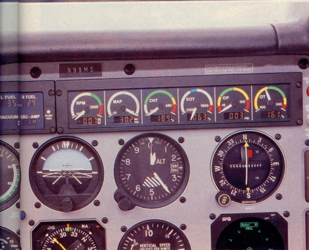
The new Moritz engine gauges show both digital and analog values (left), but the fuel, OAT, vacuum, and volt/amp gauges are only digital.
